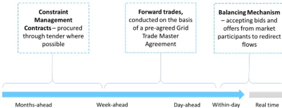
Real time transmission engineers continually monitor real time thermal constraints and transfer flows across boundaries and respond to system generated alarms and the results generated by the online power flow analysis tools. This allows our control engineers to reassess and re-optimize thermal constraint limits in real time based on the real-time system configuration, actual generation and demand. We use the Balancing Mechanism (BM) for buying flexibility from
