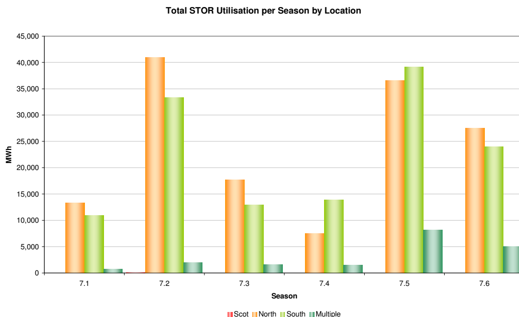
Figure 7: Total STOR energy utilisation per season by location
