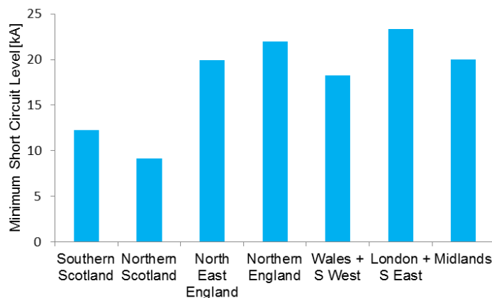
Figure 20 Minimum Short Circuit Level (2014/15)
