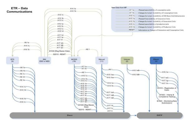
This diagram captures the flow of data and the interfaces required for the ETR solution. Data flows from each of the main actors (i.e. the Market Participants), NG Systems / Processes, external systems such as Elexon and Unicorn and any manual processes are described in more detail in our Conceptual Technical Model documentation which can be provided if required.
