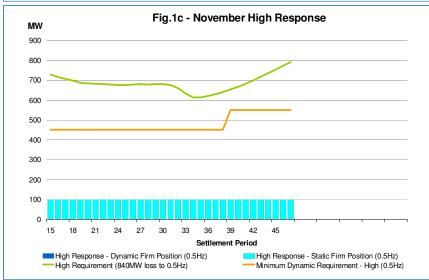
Figures 1a to 1c show the forecast frequency response requirement for each settlement period in Nov-2013.
