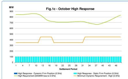
Figures 1a to 1c show the forecast frequency response requirement for each settlement period in Oct-2013.
