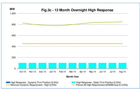
Figures 3a to 3c show the indicative night time (23:00hrs - 07:00hrs) frequency response requirement for twelve months beginning Oct-2013.
