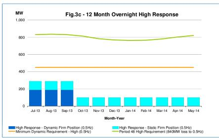
Figures 3a to 3c show the indicative daytime (23:00hrs - 07:00hrs) frequency response requirement for twelve months beginning Jul-2013.
