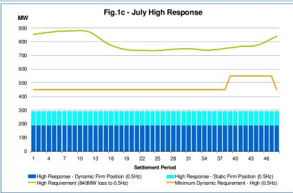
Figures 1a to 1c show the forecast frequency response requirement for each settlement period in Jul-2013.
