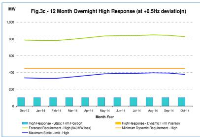
Figures 3a to 3c show the indicative night time (23:00hrs - 07:00hrs) frequency response requirement for twelve months beginning Dec-2013.
