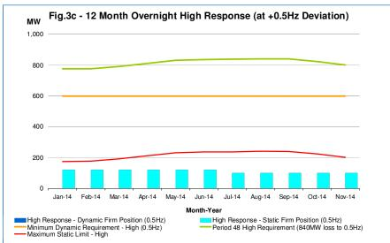
Figures 3a to 3c show the indicative daytime (23:00hrs -07:00hrs) frequency response requirement for twelve months beginning Jan-2014. The expected response requirements shown in the following graphs are averaged for each day of the month and are calculated based on the forecast demand for settlement period 48. The volume of response required will vary over individual overnight settlement periods. The figures show the base/minimum values expected overnight and assuming low wind generation.
