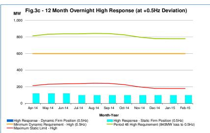
Figures 3a to 3c show the indicative daytime (23:00hrs -07:00hrs) frequency response requirement for twelve months beginning Apr-2014. The expected response requirements shown in the following graphs are averaged for each day of the month and are calculated based on the forecast demand for settlement period 48. The volume of response required will vary over individual overnight settlement periods. The figures show the base/minimum values expected overnight and assuming low wind generation.
