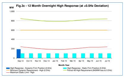
Figures 3a to 3c show the indicative daytime (23:00hrs -07:00hrs) frequency response requirement for twelve months beginning Sep-2014. The expected response requirements shown in the following graphs are averaged for each day of the month and are calculated based on the forecast demand for settlement period 48. The volume of response required will vary over individual overnight settlement periods. The figures show the base/minimum values expected overnight and assuming low wind generation.
