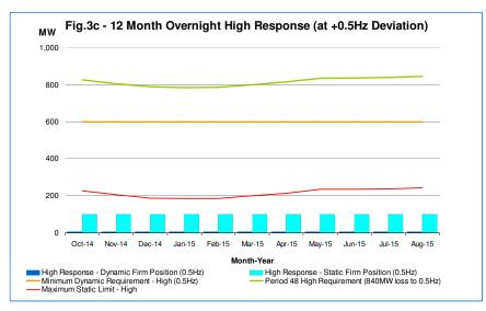
Figures 3a to 3c show the indicative daytime (23:00hrs -07:00hrs) frequency response requirement for twelve months beginning Oct-2014. The expected response requirements shown in the following graphs are averaged for each day of the month and are calculated based on the forecast demand for settlement period 48. The volume of response required will vary over individual overnight settlement periods. The figures show the base/minimum values expected overnight and assuming
