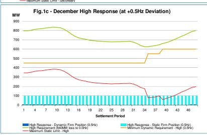
Figures 1a to 1c show the forecast frequency response requirement for each settlement period in Dec-2014.
