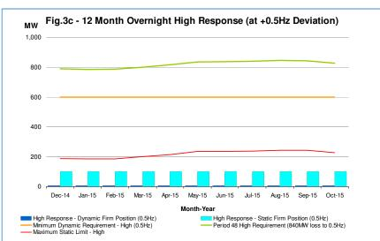
Figures 3a to 3c show the indicative daytime (23:00hrs -07:00hrs) frequency response requirement for twelve months beginning Dec-2014. The expected response requirements shown in the following graphs are averaged for each day of the month and are calculated based on the forecast demand for settlement period 48. The volume of response required will vary over individual overnight settlement periods. The figures show the base/minimum values expected overnight and assuming low wind generation.
