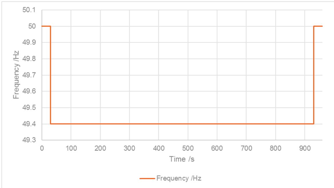
**Table 9: Test 3.1 Frequency Injection Table Corresponding with times**
