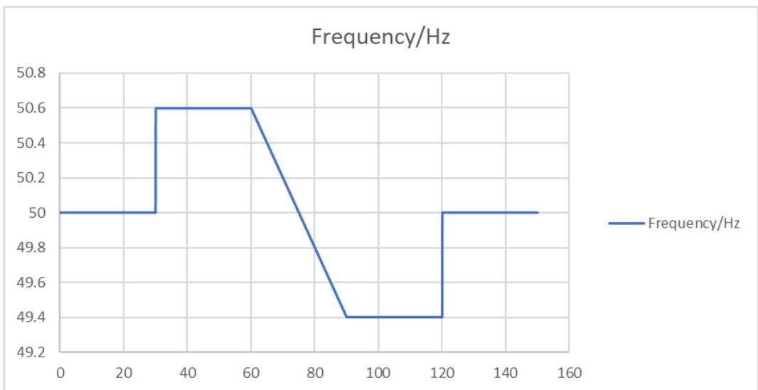
**Table 7 - Test 2 Frequency Injection Profiles**
