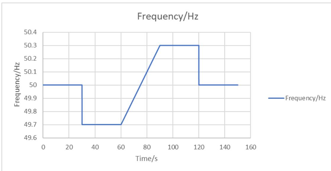
Table 14 - Test 2 Frequency Injection Profiles
