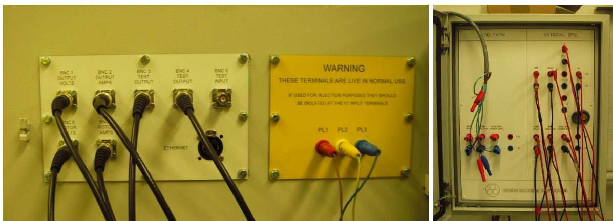
Figure 1 – Example of Compliance Test Signal Connections
