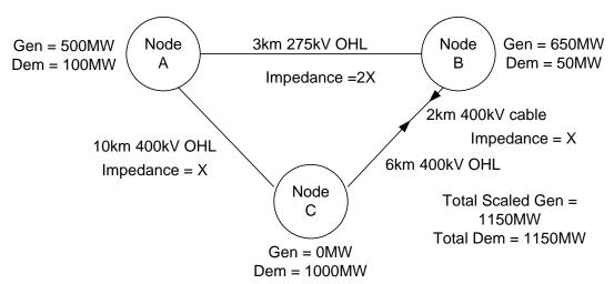
Step 2:Net export from Node B to Node C is 1000MW; route BC has impedance X and route BA-AC has impedance 3X; hence 750MW would flow down BC and 250MW along BA-AC
