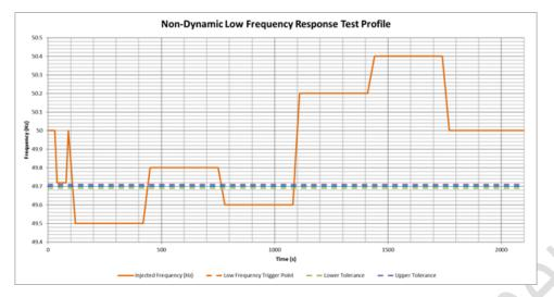
The initial frequency dip to 49.72Hz aims to prove that the relay will not activate (hence no response) if the frequency drops to just above 49.7Hz. During the sweep from 50Hz to 49.5Hz, the **Relay** should trigger at 49.7Hz (±0.01Hz). Once the **Relay** has triggered, full response should be reached within 30 seconds and be sustained for a further 1770 seconds (30 minutes after relay trigger) regardless of the varying frequency injection.
