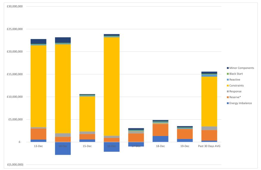
The first part of the week shows high daily costs triggered by large volume BM actions to reduce generation to manage thermal constraints due to windy weather.
