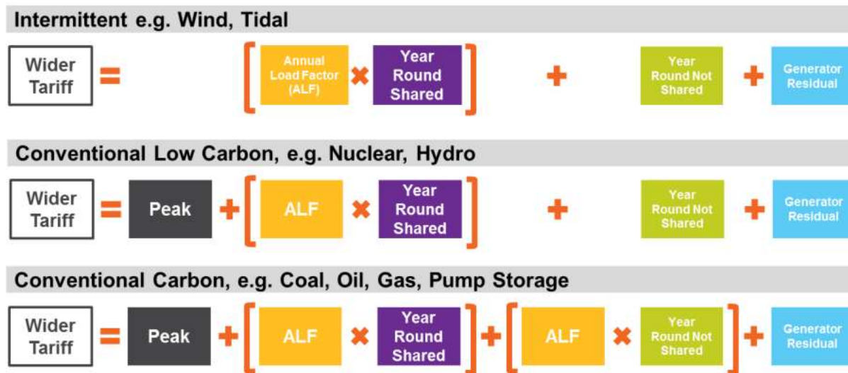
Figure 1: TNUoS Generation Classifications. See TNUoS Guidance for Generators (National Grid ESO, 2019), < https://www.nationalgrideso.com/document/138046/download >, p. 11.
