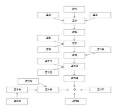
The arrows connecting generation charging zones and amalgamated generation charging zones represent the incremental km transmission boundary lengths towards the notional centre of the system. Generation located in charging zones behind arrows is considered to share based on the ratio of Low Carbon to Carbon cumulative generation TEC within those zones.
