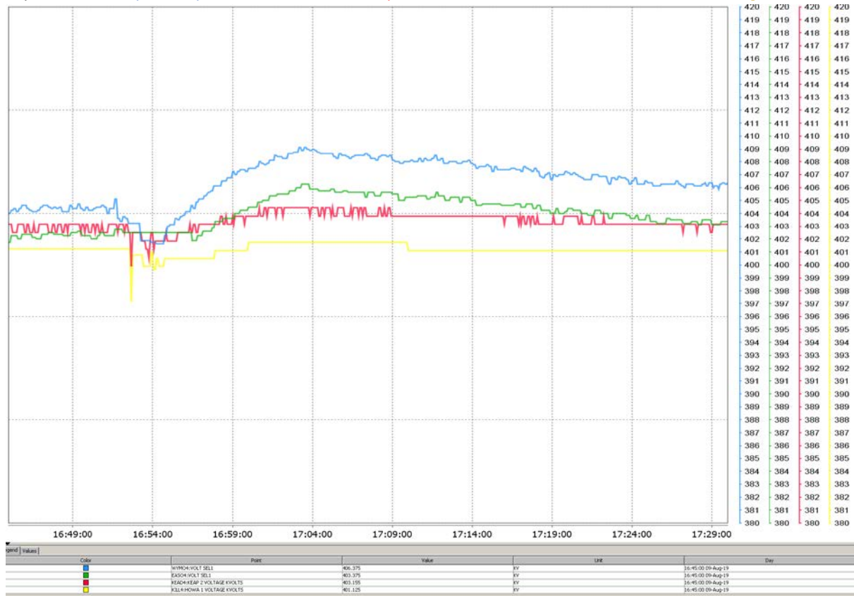
Graph 3.4 Pre-Fault and Post-Fault Steady State Voltages
