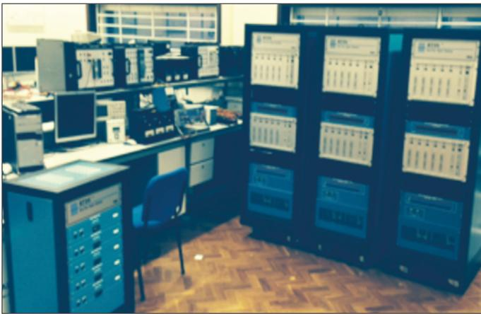
Figure 11: RTDS racks in the lab at the University of Manchester
