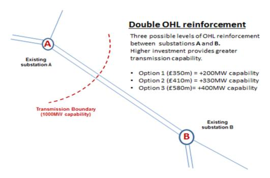
In this example, we have a transmission boundary that requires reinforcement due to changing generation background patterns. The existing network has a 1000MW capability and there are three possible reconductoring options that could be implemented. The options would provide various levels of enhancement and investment cost, as illustrated in the table below.
