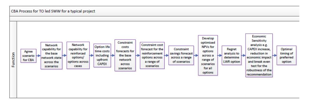
This diagram shows the overall Cost Benefit Analysis process performed for a typical new project seeking approval from Ofgem through SWW submission. Detail of the Cost Benefit Analysis methodology is explained in the Appendix C.
